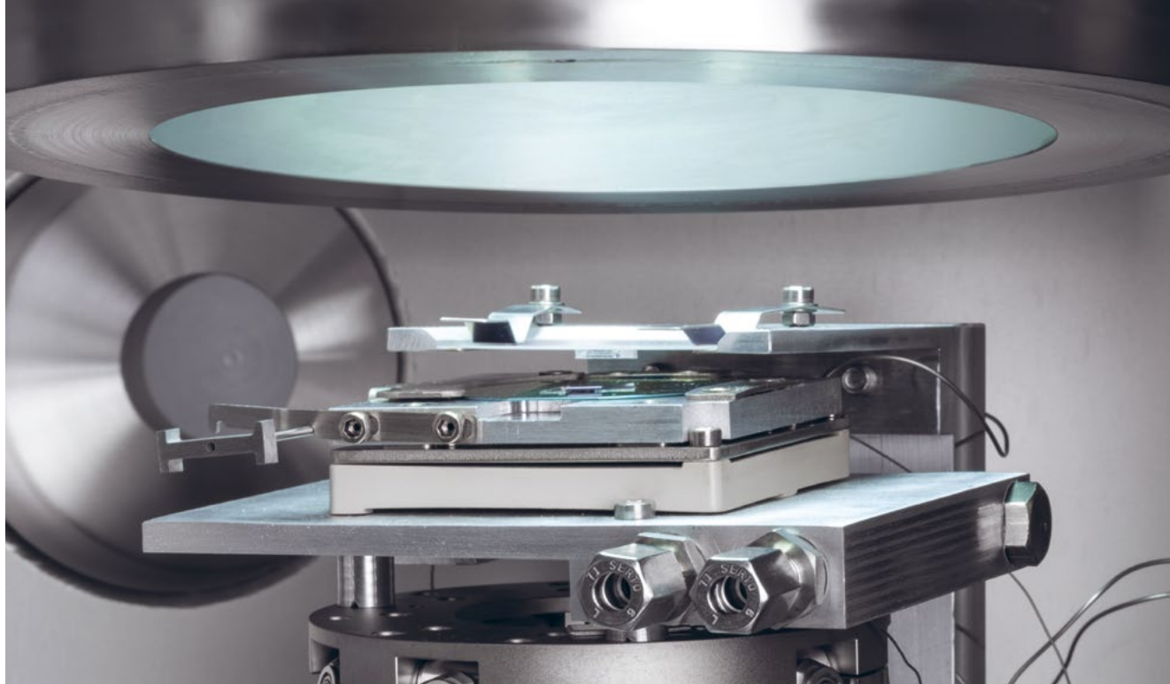
Layer transfer station to place thin crystalline membranes onto arbitrary substrates, for example 2D-MoS 2 on top of a plasmonic structure.
