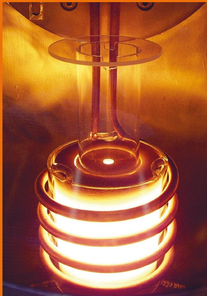
View of an AlN crystal growth experiment in progress ( T \sim 2300^\circ\text{C} ) Photo: IKZ
