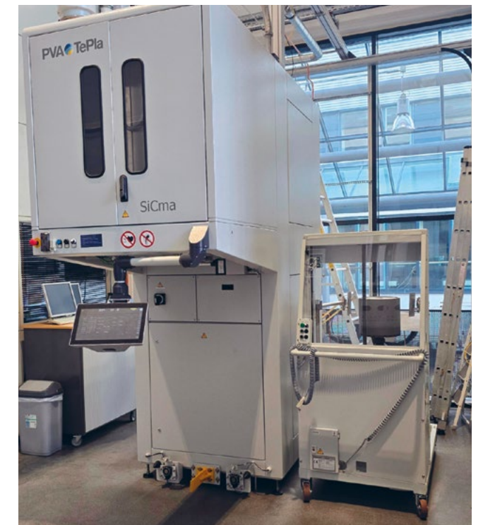
Fig. 4 AlN growth reactor from PVA TePla for AlN crystals with diameters of 100mm and beyond (installed in crystal growth hall in IKZ) Photo: IKZ
