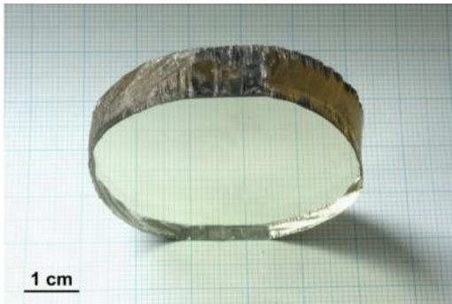
Fig. 2: Single crystal slab of Ga 2 O 3 , 2" in diameter (IKZ)
